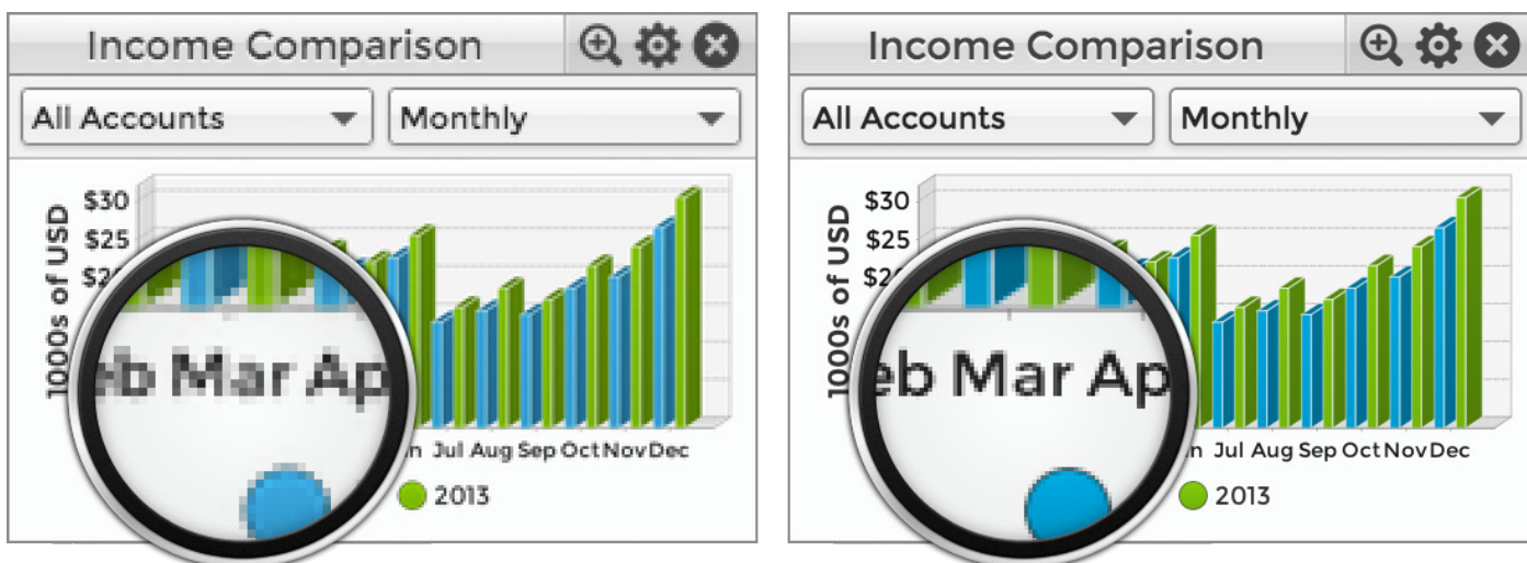
Figure 12. The dashboard on a normal display (left) and a high density display (right) that has quadruple the resolution and increased sharpness
