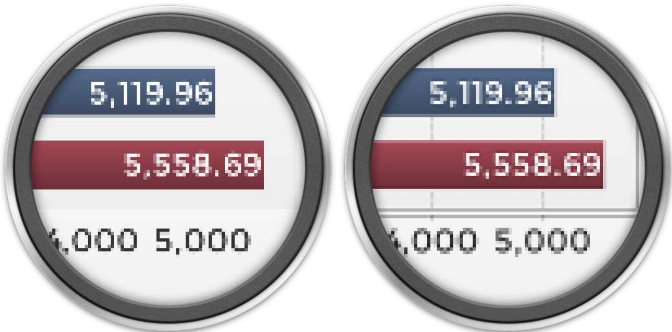
Figure 7. A comparison between scaling with Nearest Neighbor (left) and Bicubic (right) interpolations
