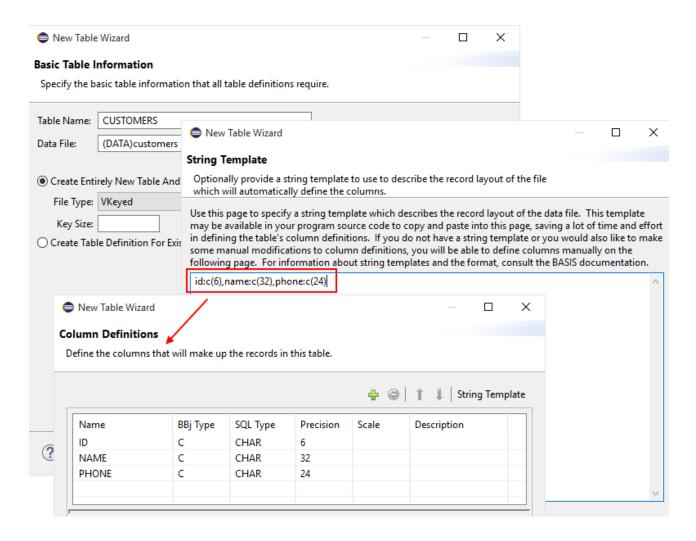
Step 2: Run the Import to Barista Dictionary utility to create the Barista element and table definitions from the import source.
