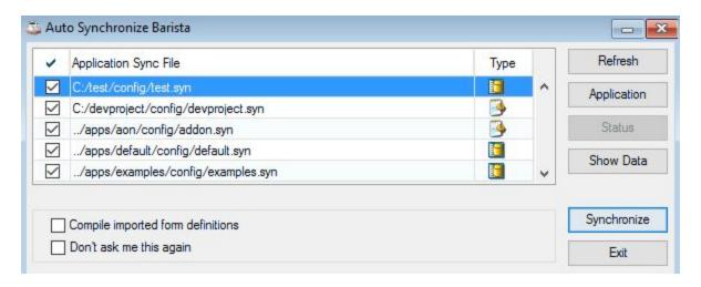
Applications not yet synchronized into the Barista data dictionary appear with a disk icon, while applications previously synchronized (if this is not a new install) have a gear or "config only" icon. In the latter case, Barista will not process all of the <application>/data/bar/\*.xml and <application>/data/cdf/\*.cdf files, but only forward data from the <application>.syn file to barista.cfg and the BASIS config.ini files.
